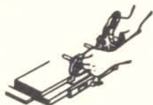
CUTTING A RABBET WITH A COMBINATION OR UNIVERSAL PLANE
